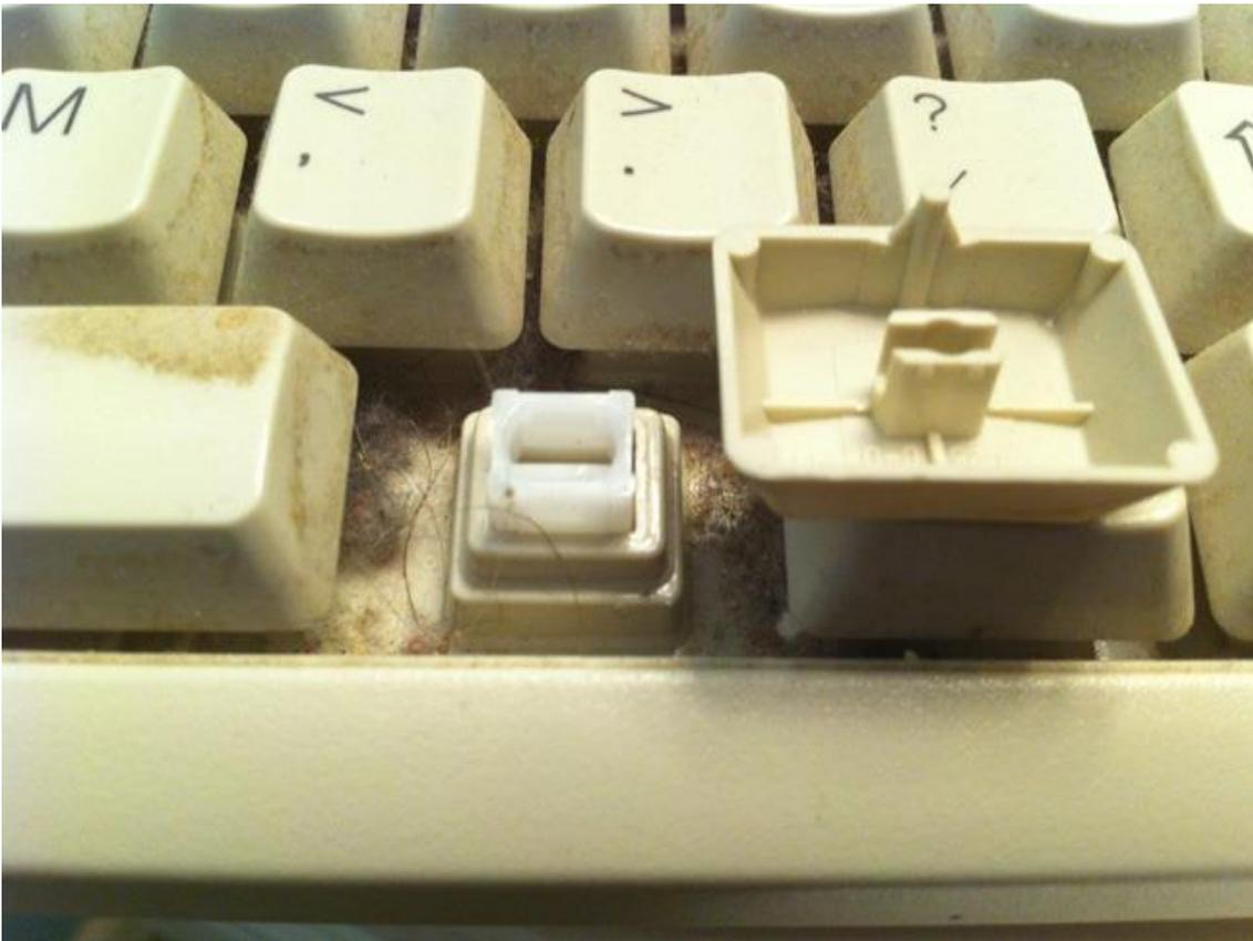
For laptop keyboards, your fingernail should be enough to pull the plastic up. Start with one corner and move to an adjacent one. Be extra careful, since the mechanism is made of plastic and you don't want to break it.
